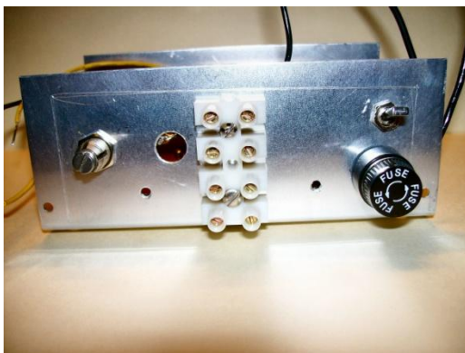
Front of partially assembled power supply
